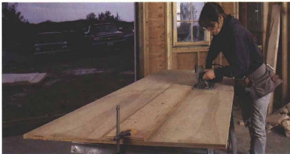
A strip of plywood serves as a guide for cutting wide pieces.
