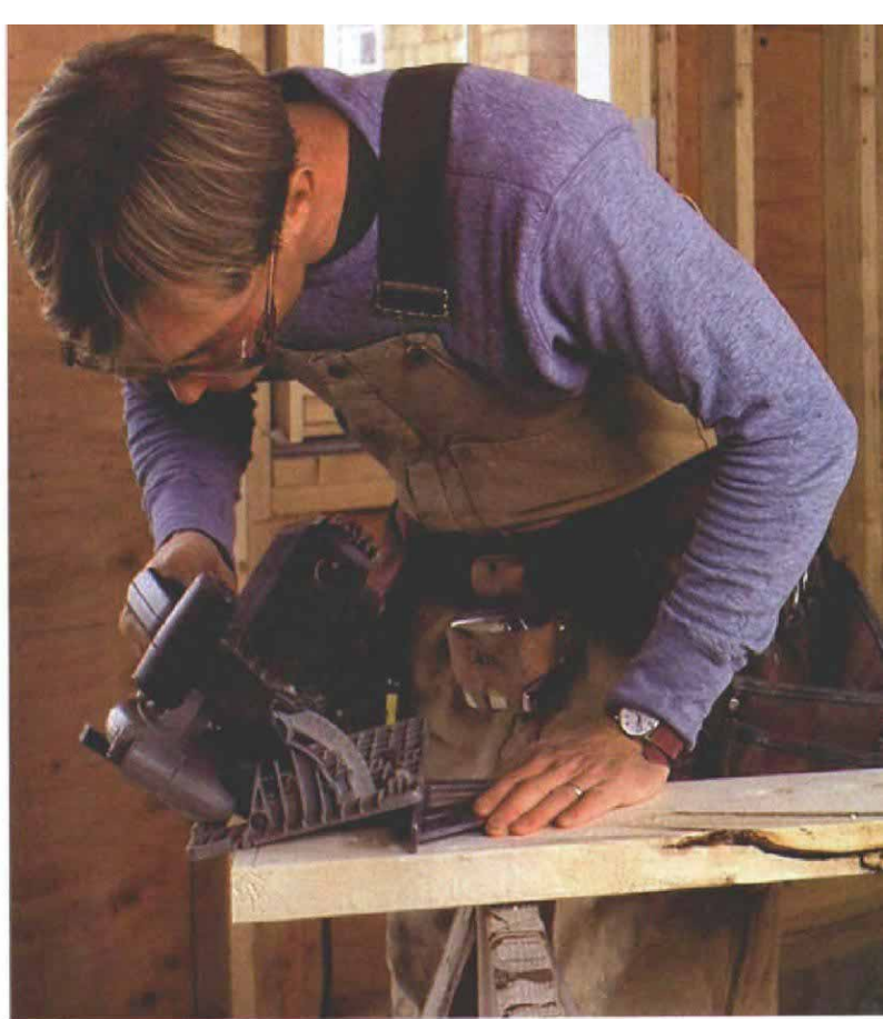
Lifting the saw base lets you cut angles beyond 45°.
