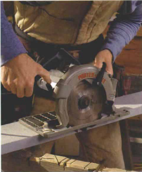
Blade depth is set \frac{1}{8} in. beyond work
