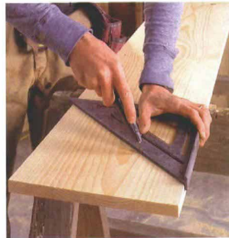
Prescoring the cut reduces splintering.
