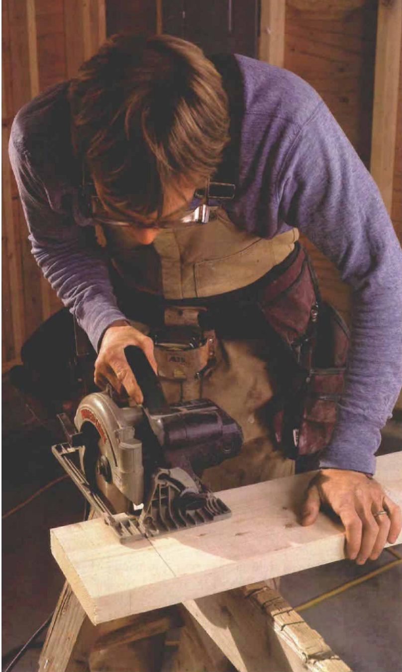
Start with the blade and the saw-base notch on the line.
