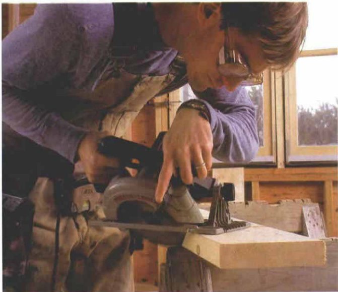
Hold the guard up so that it won't jam on compound miters.
