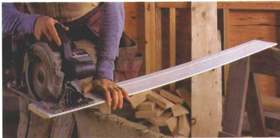
Cutting from the backside puts the smoothest side of the cut on the finished face.
